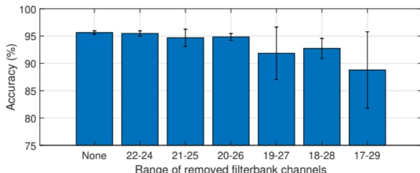
$$f_{k=23} \approx 2,000 \text{ Hz}, \quad [20, 26] \equiv [1,626, 2,564] \text{ Hz}$$
